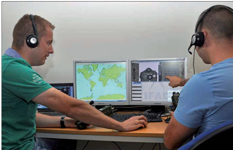
The real 152 radio is compared to its simulated counterpart. The radio simulator is developed by IFAD TS, a training developed by IFAD TS, a training simulation software company based in Odense, Denmark.
